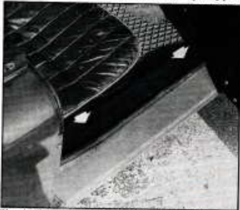
Chassis side members do rust, so pull back the carpets (arrows) and check along each side carefully
