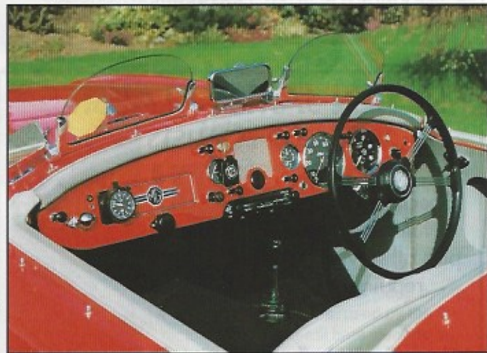
Tell-tale rev counter dominates dash. Note horn and additional rear view mirror on co-drivers side. Grey trim and hood contrasts well.
